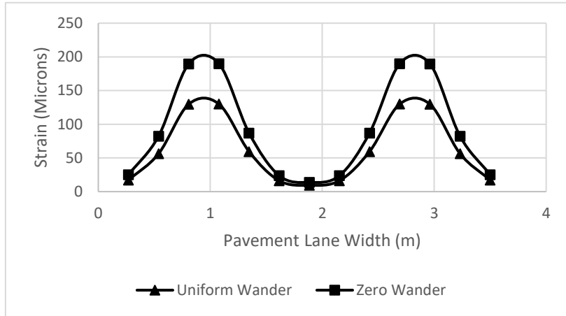
Fig. 9-15: Class-1 truck strain values with zero wander and uniform wander
