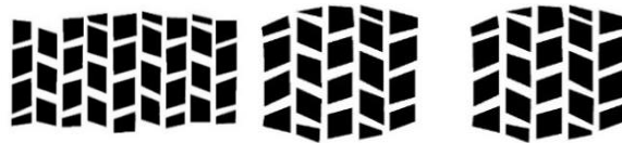
Fig. 7-3: Wide (left) and dual (right) tire footprint.
