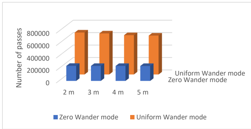
Fig. 9-26: Number of passes to reach rut depth value of 6 mm under various lateral wander modes and headway distance values.
